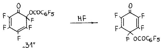
Perfluoro 4-phenoxy-2,5-cyclohexadien-1-one "23" remains unchanged in the reaction with HF at 20° [49], whereas perfluoro-6-phenoxy-2,4-cyclohexadien-1-one is isomerised with migration of both the fluorine atom and the pentafluorophenoxy group. These two processes seem to follow different mechanisms:
